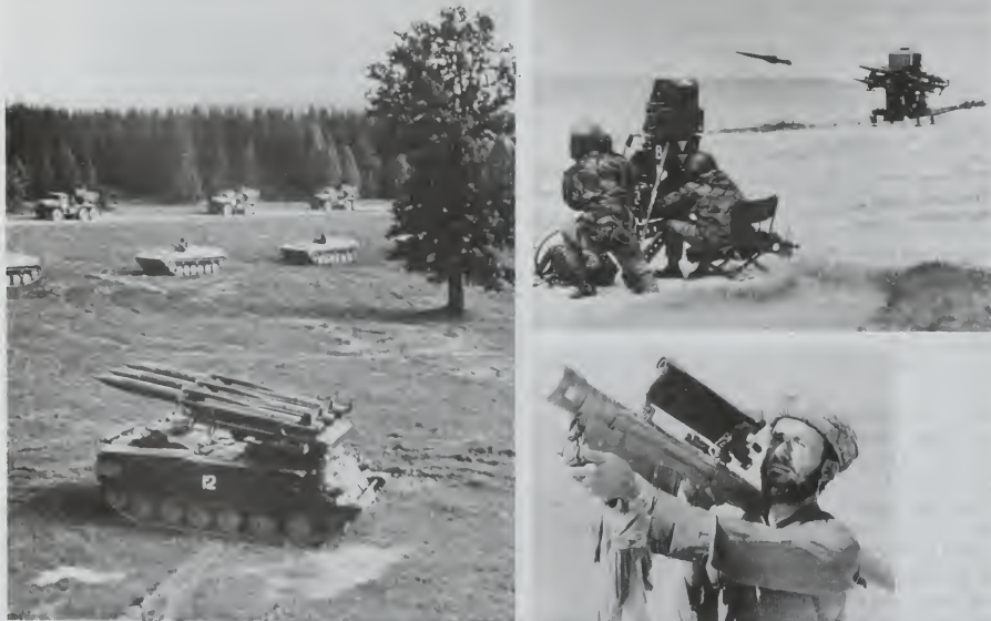
Figure 18: Three mobile surface-to-air missiles, for low- and medium-level anti-aircraft defense. (Left) The SA-6 Gainful (built by the former U.S.S.R.), tracked and guided by radar, on maneuvers with armored personnel carriers and truck-mounted artillery rockets. (Top right) The optically tracked and radio-guided version of the British Rapier, as deployed in the Falkland Islands. (Bottom right) The infrared-homing U.S. Stinger, in the hands of an Afghan guerrilla fighter.
